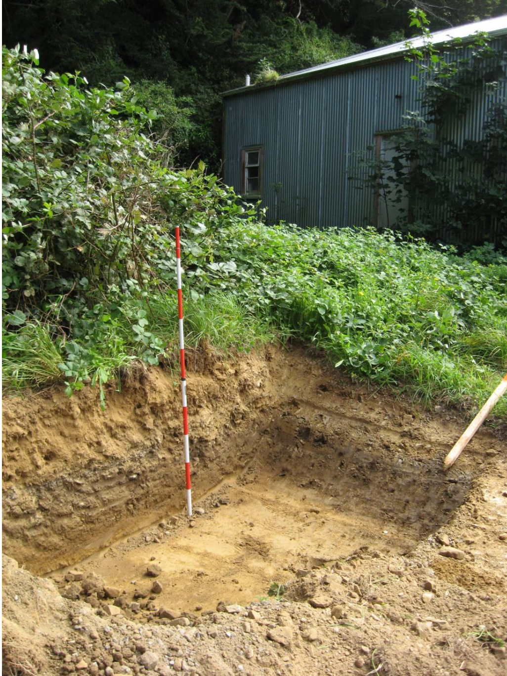
Fig. 4. Engineers' test pit February 2011 showing yellow-brown subsoil and original grey loam topsoil overlain by yellow-brown fill from clearance of the building platform.
