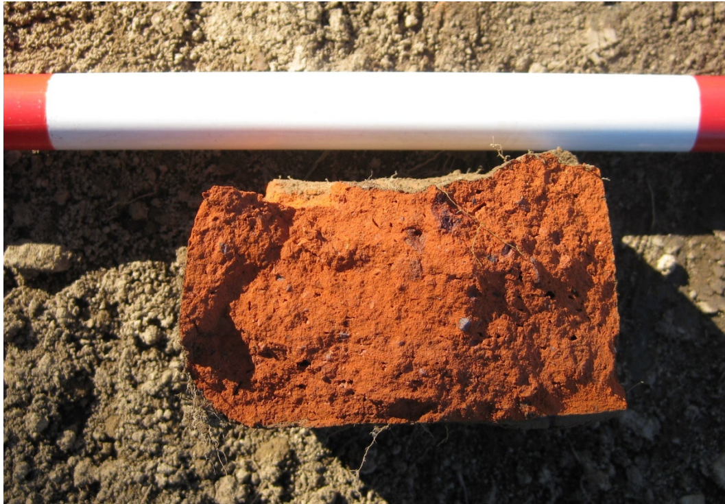
Fig. 24. Sections through bricks, showing orange poorly fired fabric, frogged brick at bottom. Scale bar 20 cm.
