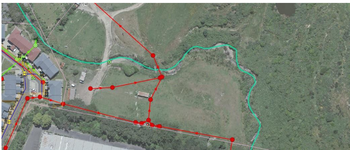
Figure 2. Sewage pipe network (in red).
